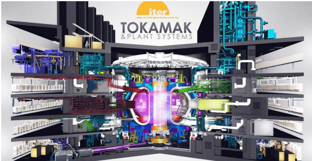
Figure 2: Cut away diagram of the ITER device being built in Cadarache, France (source: ITER Organization)
